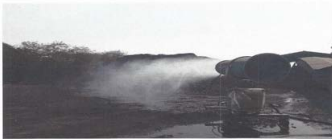
Typical view of Mobile dust suppression system installed at TPP & Limestone pile
